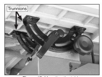
Figure 17. Mounting the table.
